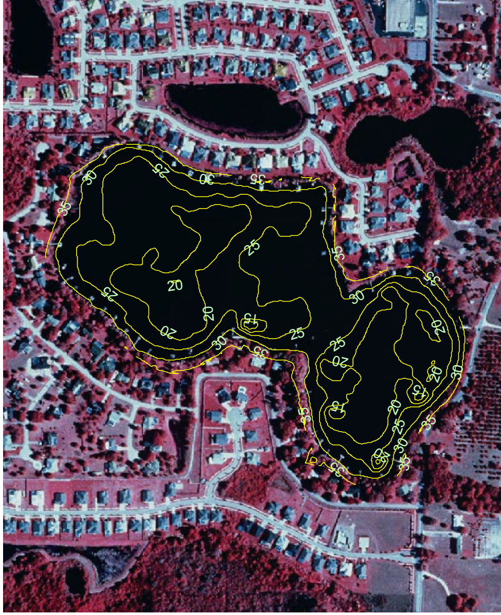
Figure Fairy-3. Five-foot contours within the Fairy Lake basin in Hillsborough County, Florida. Values shown are elevations, in feet, above the National Geodetic Vertical Datum of 1929.
